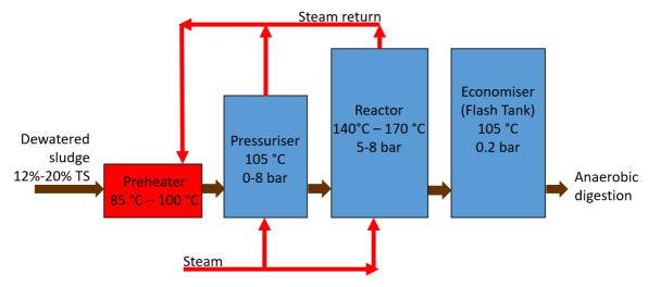
Example for a thermal hydrolysis process with high pressure
