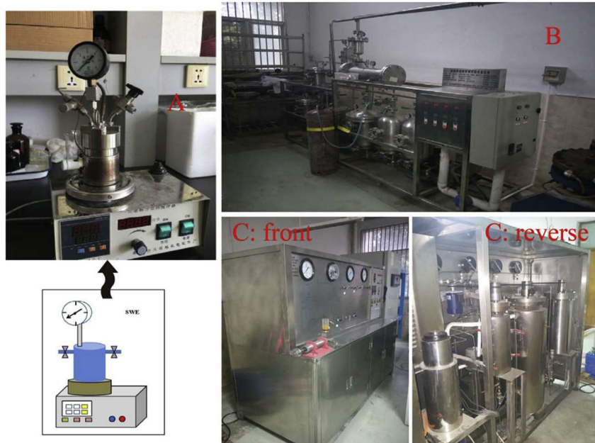
Figure 4 Simple static equipment of SWE in laboratory (A); industrial dynamic equipment of SWE (B, C) (Zhang et al., 2020).
