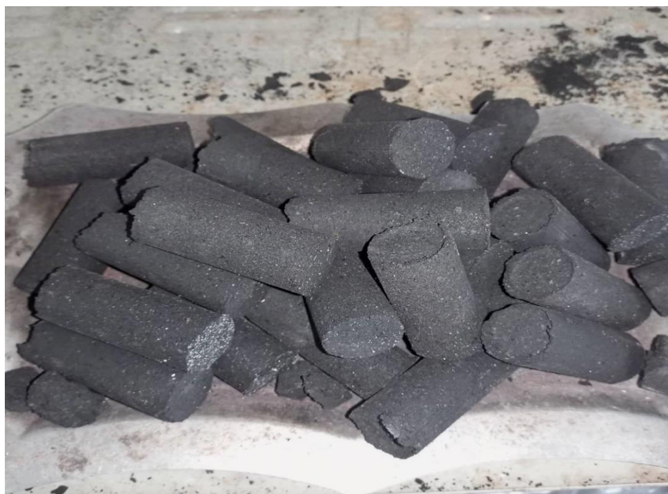
Figure 10: Laboratory produced biochar using different ratios of sludge and saw dust
