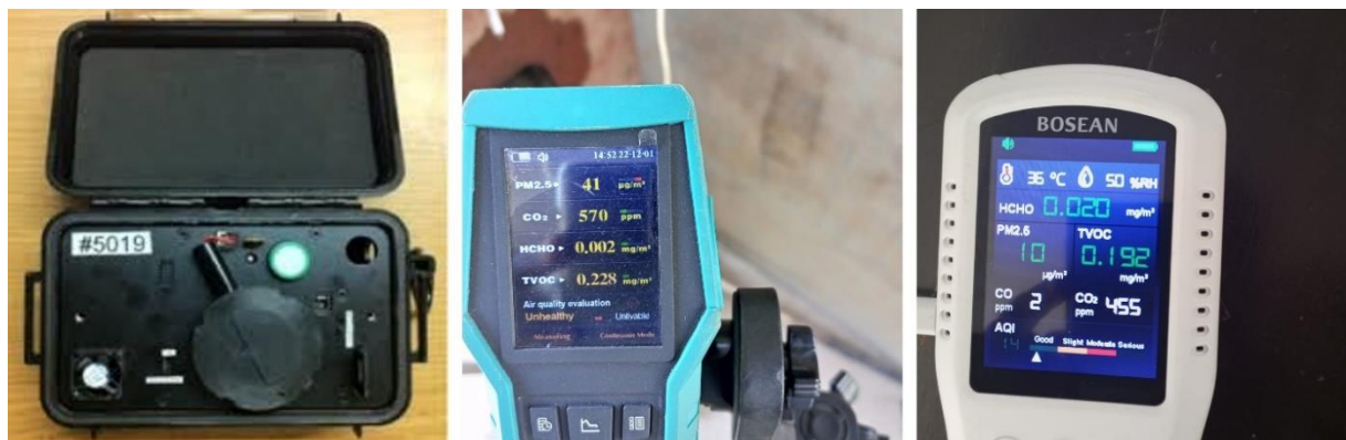
Figure 12: Air monitoring meters used for monitoring air quality. Left meter is the Aprovecho IAP used in measuring personal exposure of the cook to CO and PM 2.5 during the use of the biochar.
