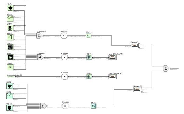
\*Inline loggers operate the same as normal loggers, but let the signal pass through.
