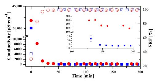
**Figure 4.** Permeate conductivity and SRF in an operation day with the AS7 module (blue squares and blue empty squares respectively) and the AS24 module (red circles and red empty circles respectively) both in AGMD configuration.
