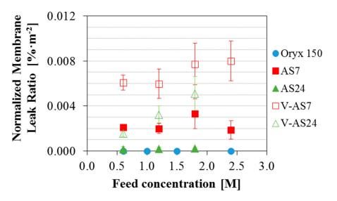
**Figure 7.** Normalized Membrane Leak Ratio obtained with the Oryx 150, the AS7 and the AS24 modules (in AGMD and V-AGMD configuration) for different initial feed concentrations.  $T_{hot} = 80$  °C;  $T_{cold} = 25$  °C; F = 1100 L·h<sup>-1</sup> (AS modules) and 600 L·h<sup>-1</sup> (Oryx 150).
