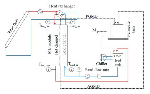
Figure 1. Process flow diagram of the membrane distillation (MD) operation.
