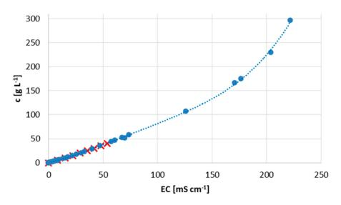
**Figure A1.** Salt concentration as a function of electrical conductivity. Blue dots: NaCl aqueous solution. Red crosses: seawater.
