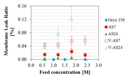
**Figure 6.** Membrane Leak Ratio obtained with the Oryx 150, the AS7 and the AS24 modules (in AGMD and V-AGMD configuration) for different initial feed concentrations.  $T_{hot} = 80$  °C;  $T_{cold} = 25$  °C;  $F = 1100 \text{ L}\cdot\text{h}^{-1}$  (AS modules) and 600 L·h<sup>-1</sup> (Oryx 150).
