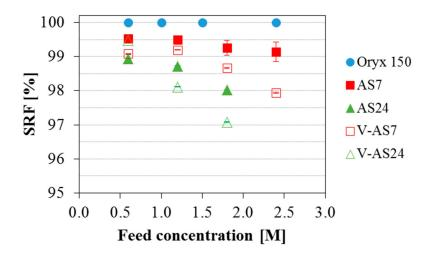
**Figure 5.** SRF obtained with the Oryx 150, the AS7 and the AS24 modules (in AGMD and V-AGMD configurations) for different initial feed concentrations.  $T_{hot} = 80 \text{ °C}$ ,  $T_{cold} = 25 \text{ °C}$  and  $F = 1100 \text{ L} \cdot \text{h}^{-1}$  (AS modules) and 600 L $\cdot$ h<sup>-1</sup> (Oryx 150).
