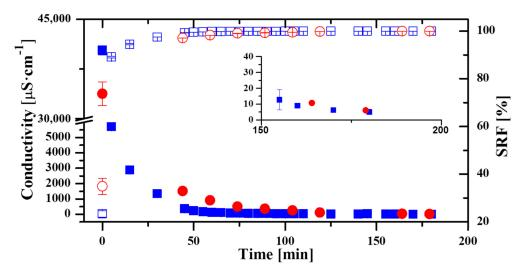
**Figure 2.** Permeate conductivity and Salt Rejection Factor (SRF) obtained in two typical days of operation with the module Oryx 150. Blue squares: conductivity of day 1; red circles: conductivity of day 2; blue empty squares: SRF of day 1; red empty squares: SRF of day 2.
