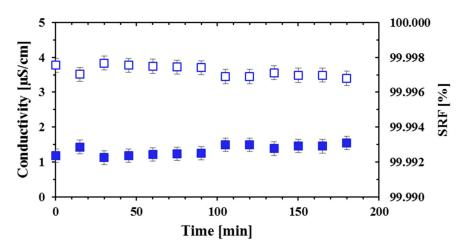
**Figure 3.** Permeate conductivity and SRF obtained with the module Oryx 150 after cleaning with demineralized water at 80 °C. Blue squares: conductivity, blue empty squares: SRF.
