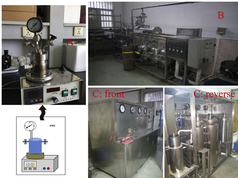
Fig. 4. Simple static equipment of SWE in laboratory (A); industrial dynamic equipment of SWE (B, C) produced by Jiangsu University.
